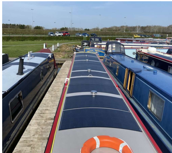
12 x 160W (1920W) Solar Panels
